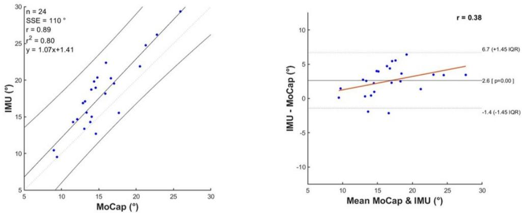
Figure 9. Results from the linear regression, Pearson correlation, and Bland-Altman analyses for all chest pass static throws performed.
