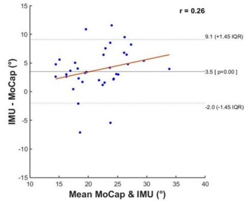
Figure 12. Results from the linear regression, Pearson correlation, and Bland-Altman analyses for all rotational static throws performed.
