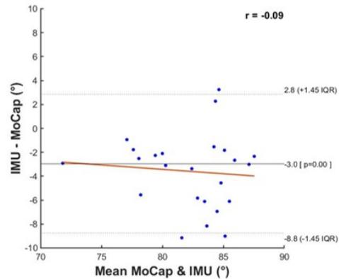
Figure 15. Results from the linear regression, Pearson correlation, and Bland-Altman analyses for all vertical static throws performed.
