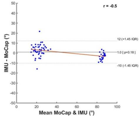
Figure 5. Results from the linear regression, Pearson correlation, and Bland-Altman analyses for all throws performed at sub-maximal intensity.
