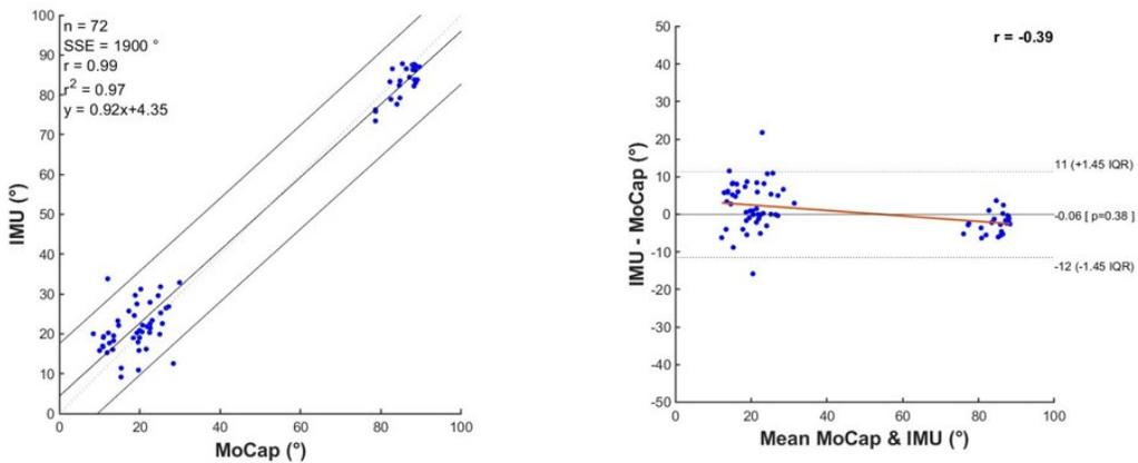
Figure 4. Results from the linear regression, Pearson correlation, and Bland-Altman analyses for throws performed at maximal intensity.
